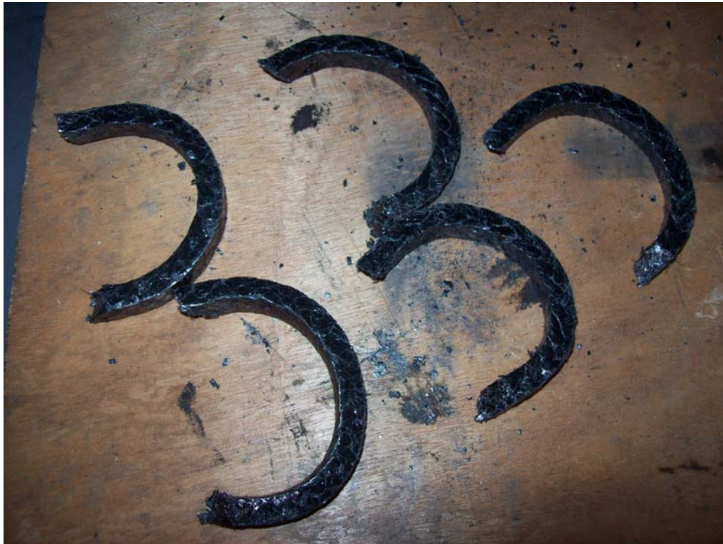
Packing Material – Rings cut and installed by Matt Wasielewski, Yarmouth
