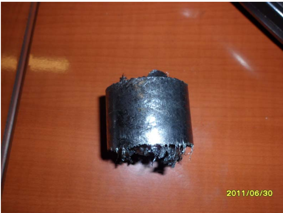
Packing rings after test
